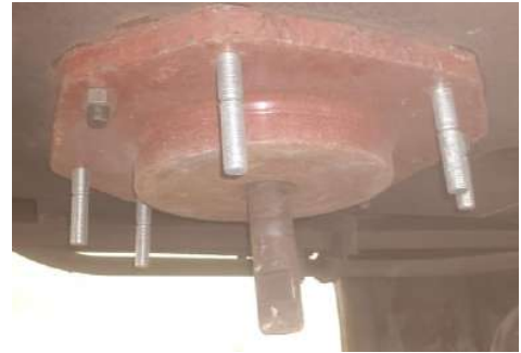
Figure 21 Flat CP top locating at mounting face (02 bolts shall be fitted diagonally opposite to hold the pivot in its position)
