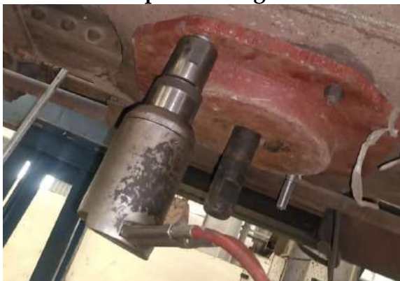
Figure 22 New Flat CP top fitment (Lock bolting shall be done in remaining 04 holes with fitment in diagonally opposite location in sequence, removal of holding bolts and lock bolting in these two holes)
