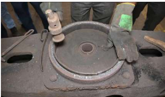
Figure 8 Flat CP- new liner fitment (marking shall be on non-wearing surface)
