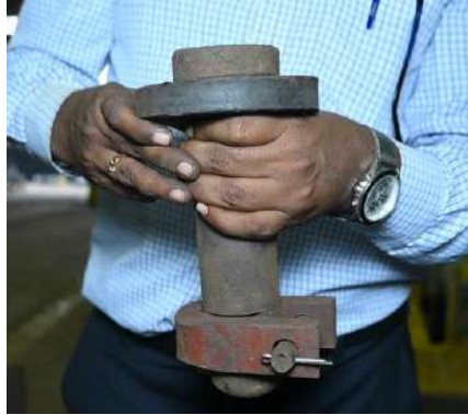
Figure 26 CP pin assembly
