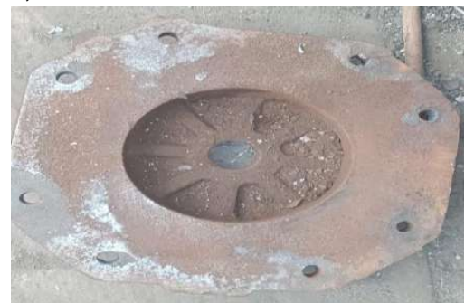
Figure 18 Flat CP top removal (Flat CP top removal (Rivet/lock bolt shall be cut using gas torch and damage to body bolster should be avoided. Care shall be also be taken to avoid any injury, due to falling of top CP)
