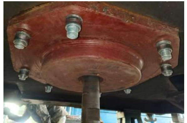
Figure 25 New Flat CP top fitment (Lock bolting shall be done in remaining 04 holes with fitment in diagonally opposite location in sequence, removal of holding bolts and lock bolting in these two holes)
