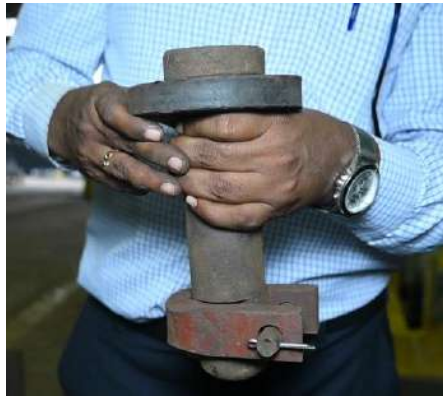
Figure 17 CP pin assembly
