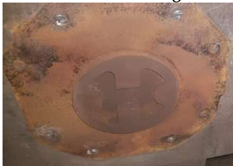
Figure 33 Flat CP top mounting location examination- Surface shall be examined for any crack etc. and attended as per relevant repair procedure of body bolster of the respective wagon Figure 34 Flat CP top locating at mounting face (2 bolts shall be fitted diagonally opposite to hold the pivot in its position)
