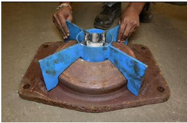
Figure 11 New Spherical CP top gauging before fitment (3 mm filler gauge must not pass at time of fitment)
