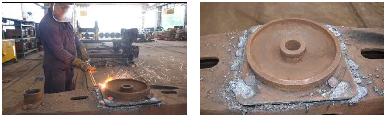
Figure 5 Spherical CP bottom removal (flame shall be pointed towards CP bottom to avoid damage to bolster)
