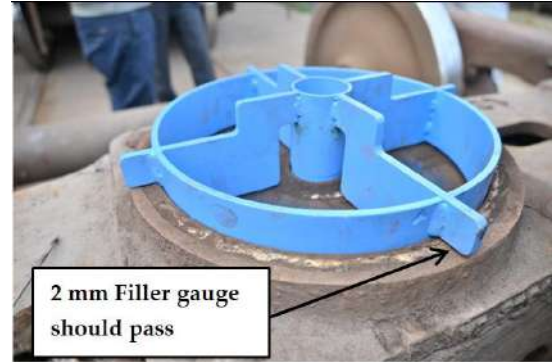
Figure 13 Flat CP- vertical gauging after liner fitment (gauge should rotate without any obstruction to ensure proper fitment)
