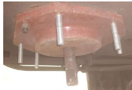
Figure 31 Flat CP top locating at mounting face (2 bolts shall be fitted diagonally opposite to hold the pivot in its position)
