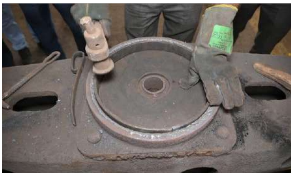
Figure 5 Flat CP- new liner fitment (marking shall be on non-wearing surface)
