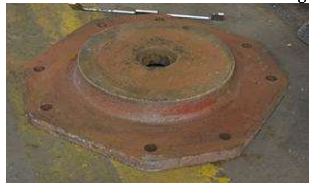
Figure 22 New Flat CP top examination (Gauge should rotate without any obstruction and 2 mm filler gauge must not pass between gauge and CP on horizontal and vertical surfaces at the time of fitment)
