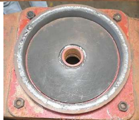
Figure 26 New flat CP bottom fitment with liners (Two bolts shall be fitted diagonally to hold the CP in position, followed by riveting in two holes, removal of bolts and riveting in remaining two holes followed by welding of CP bottom with bogie bolster)
