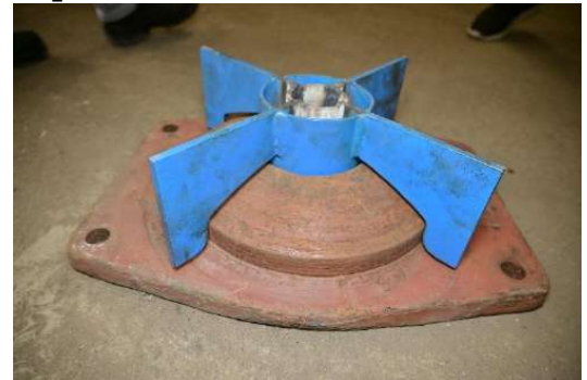
Figure 23 Spherical CP top examination (gauge no. WD-25094-S/2 should rotate freely over CP top)
