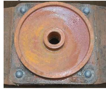
Figure 21 Welding of CP bottom with bogie bolster
