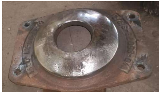
Figure 22 Spherical CP top removal (Rivet/lock bolt shall be cut using gas torch, damage to body bolster should be avoided. Care shall be also be taken to avoid any injury, due to falling of top CP)
