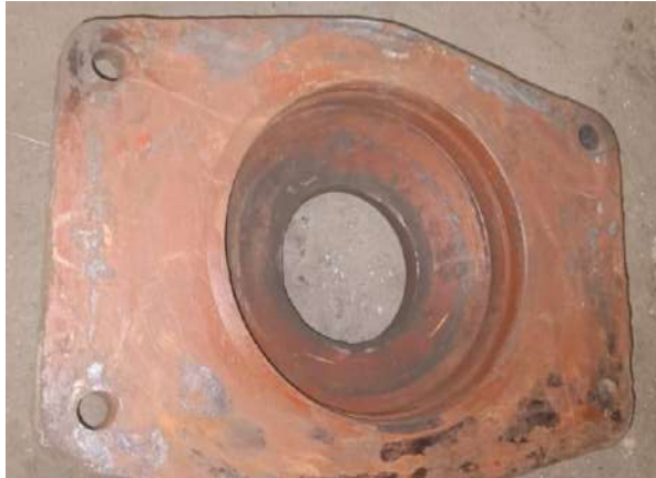
Figure 13 Spherical CP top examination (gauge no. WD-25094-S/2 should rotate freely over CP top)
