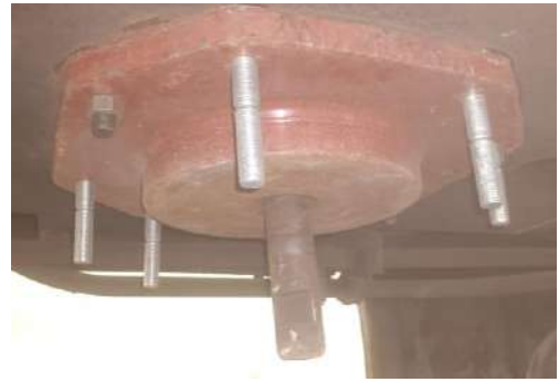
Figure 24 Flat CP top locating at mounting face (02 bolts shall be fitted diagonally opposite to hold the pivot in its position)
