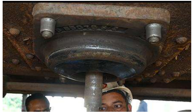
Figure 16 Spherical CP top fitment (two diagonal holding bolts shall be fitted, followed by lock bolting in two holes, subsequent removal of holding bolt and lock bolting in these two holes)
