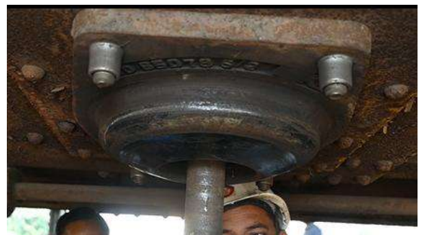
Figure 26 Spherical CP top fitment (two diagonal holding bolts shall be fitted, followed by lock bolting in two holes, removal of holding bolt and lock bolting, one at a time in the remaining two holes)
