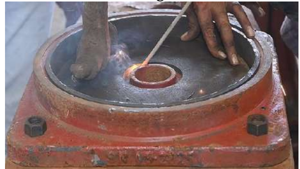
Figure 25 flat CP bottom removal (flame shall be pointed towards CP bottom to avoid damage to bolster)
