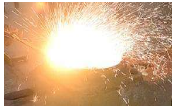
Figure 28 flat CP bottom removal (flame shall be pointed towards CP bottom to avoid damage to bogie bolster)
