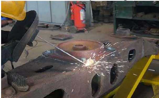
Figure 21 Welding of CP bottom with bogie bolster
