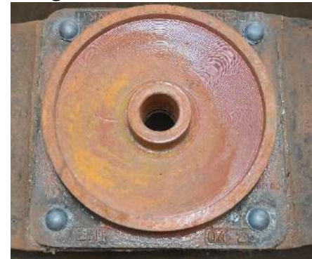
Figure 7 Welding of CP bottom with bogie bolster
