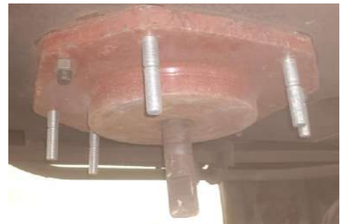
Figure 33 Flat CP top mounting location examination- Surface shall be examined for any crack etc. and attended as per relevant repair procedure of body bolster of the respective wagon Figure 34 Flat CP top locating at mounting face (2 bolts shall be fitted diagonally opposite to hold the pivot in its position)
