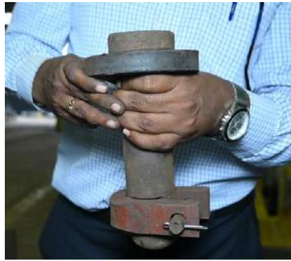
Figure 17 CP pin assembly
