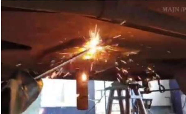
Figure 12 Spherical CP top removal (Rivet/lock bolt shall be cut using gas torch and damage to body bolster should be avoided. Care shall also be taken to avoid any injury, due to falling top CP)
