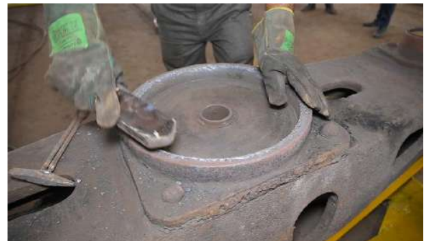
Figure 4 Flat CP- cleaning after liner removal
