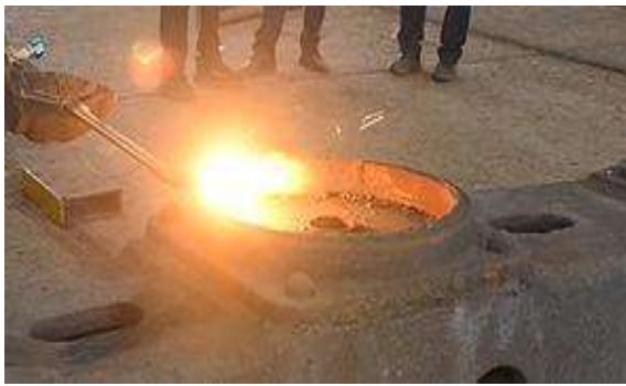
Figure 28 flat CP bottom removal (flame shall be pointed towards CP bottom to avoid damage to bogie bolster)
