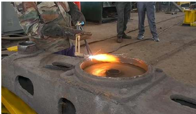
Figure 3 Flat CP liner removal (Damage to CP should be avoided)
