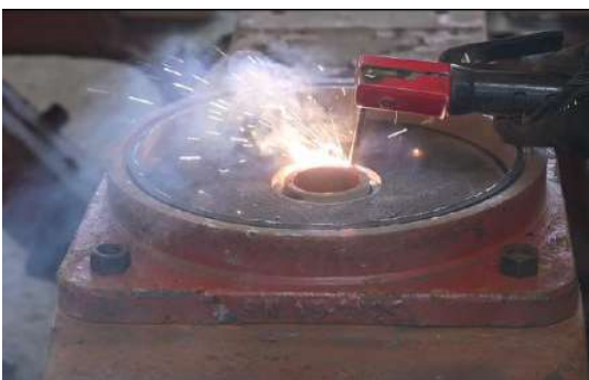
Figure 9 Flat CP- horizontal liner complete welding all along the periphery as per drawing. Post welding top surface of liner should be free from any burrs, weld projection etc. which shall be grinded
