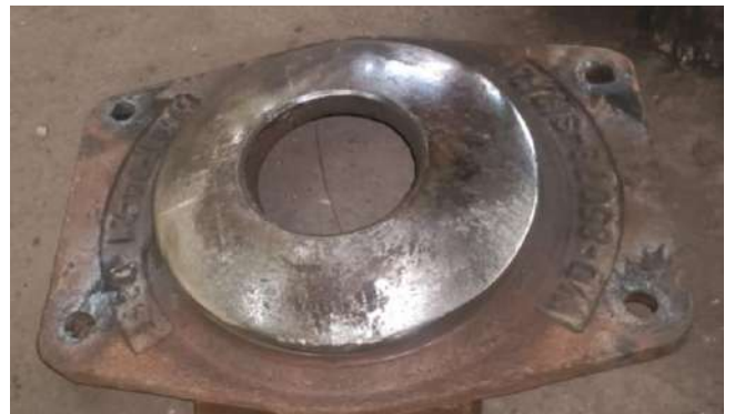
Figure 22 Spherical CP top removal (Rivet/lock bolt shall be cut using gas torch and damage to body bolster should be avoided. Care shall also be taken to avoid any injury, due to falling of top CP)
