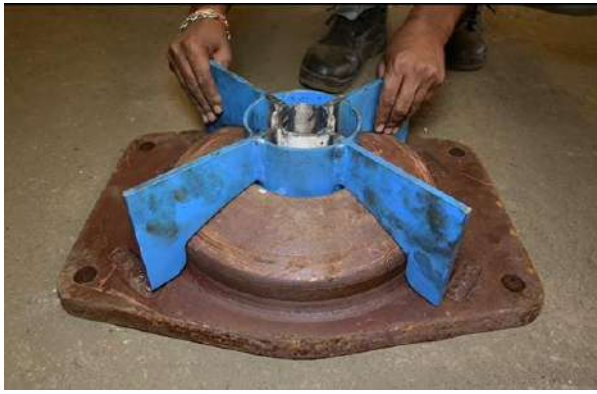
Figure 11 New Spherical CP top gauging before fitment (3 mm filler gauge must not pass at the time of fitment)
