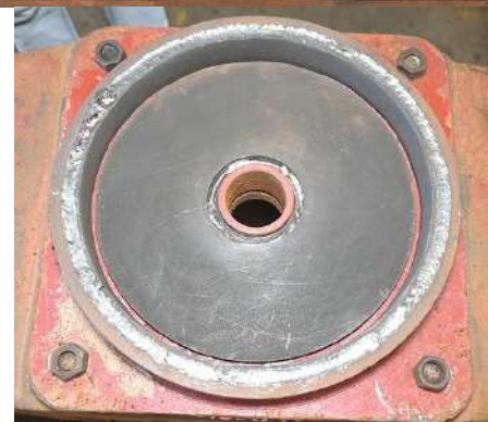
Figure 29 New flat CP bottom fitment with liners (Two bolts shall be fitted diagonally to hold the CP in position, followed by riveting in two holes, removal of bolts and riveting in remaining two holes followed by welding of CP bottom with bogie bolster)
