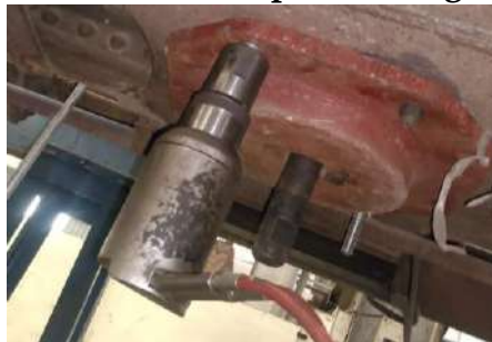
Figure 32 New Flat CP top fitment (Lock bolting shall be done in remaining 04 holes with fitment in diagonally opposite location in sequence, removal of holding bolts and lock bolting in these two holes)
