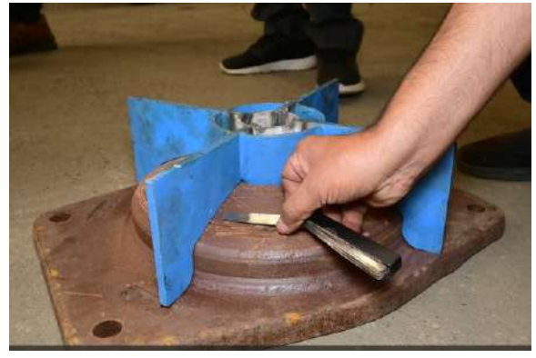
Figure 11 New Spherical CP top gauging before fitment (3 mm filler gauge must not pass at the time of fitment)
