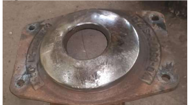
Figure 12 Spherical CP top removal (Rivet/lock bolt shall be cut using gas torch and damage to body bolster should be avoided. Care shall also be taken to avoid any injury, due to falling top CP)
