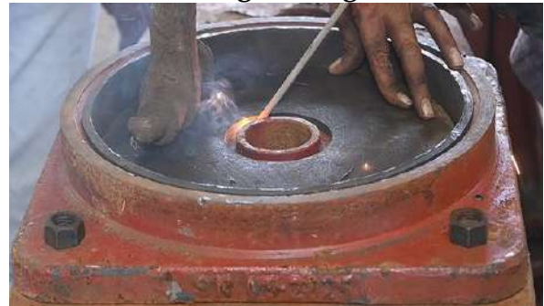
Figure 28 flat CP bottom removal (flame shall be pointed towards CP bottom to avoid damage to bogie bolster)
