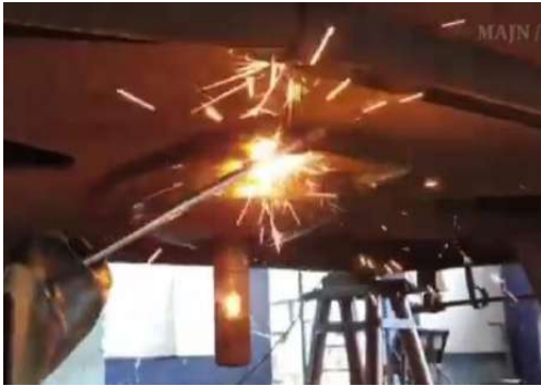
Figure 31 Flat CP top removal (Rivet/lock bolt shall be cut using gas torch and damage to body bolster should be avoided. Care shall be also be taken to avoid any injury, due to falling of top CP)
