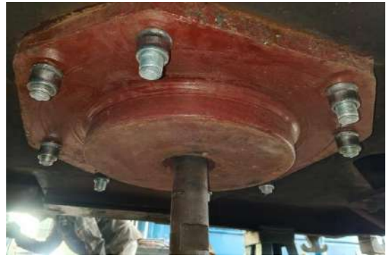
Figure 35 New Flat CP top fitment (Lock bolting shall be done in remaining 04 holes with fitment in diagonally opposite location in sequence, removal of holding bolts and lock bolting in these two holes)
