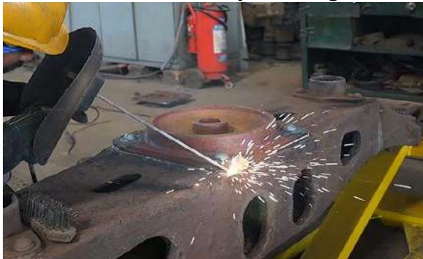
Figure 7 Welding of CP bottom with bogie bolster
