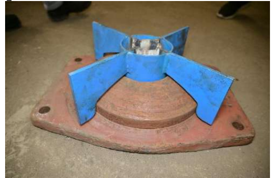
Figure 23 Spherical CP top examination (gauge no. WD-25094-S/2 should rotate freely over CP top)
