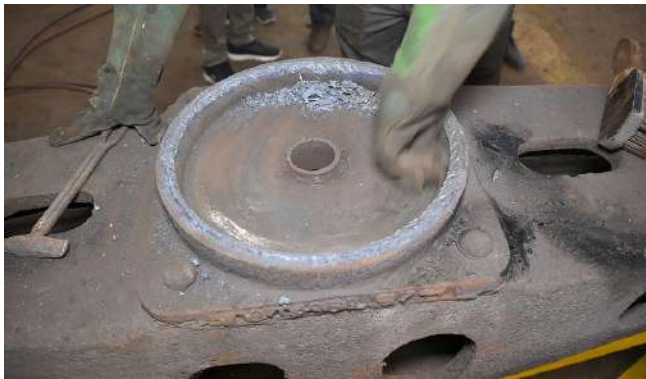
Figure 1 Flat CP bottom cleaning
