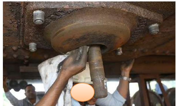
Figure 2 Spherical CP Top shall be removed for examination of body bolster area
