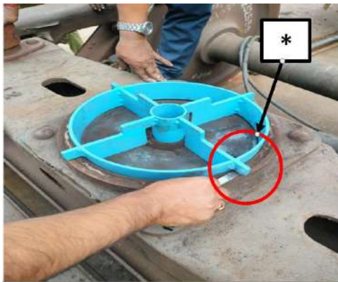
Figure 4 Checking of Vertical wear (Wear on Horizontal Liner)
