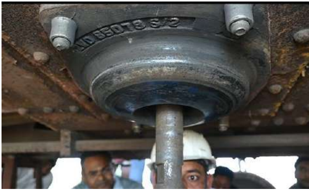
Figure 16 Spherical CP top fitment (two diagonal holding bolts shall be fitted, followed by lock bolting in two holes, subsequent removal of holding bolt and lock bolting in these two holes)
