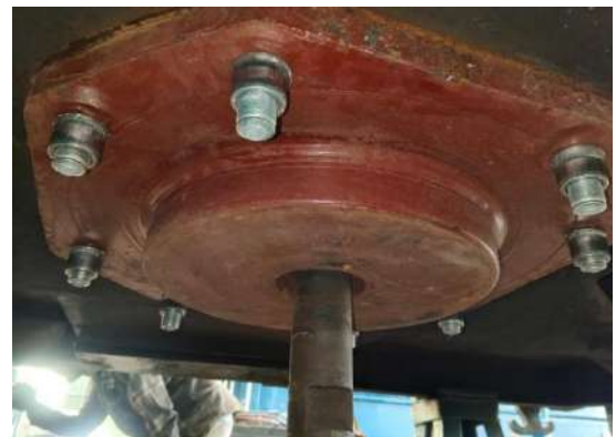
Figure 22 New Flat CP top fitment (Lock bolting shall be done in remaining 04 holes with fitment in diagonally opposite location in sequence, removal of holding bolts and lock bolting in these two holes)
