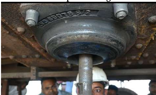
Figure 26 Spherical CP top fitment (two diagonal holding bolts shall be fitted, followed by lock bolting in two holes, removal of holding bolt and lock bolting, one at a time in the remaining two holes)
