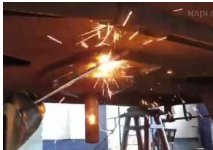
Figure 28 Flat CP top removal (Rivet/lock bolt shall be cut using gas torch and damage to body bolster should be avoided. Care shall be also be taken to avoid any injury, due to falling of top CP)
