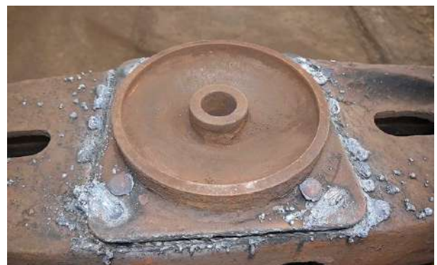
Figure 19 Spherical CP bottom removal (flame shall be pointed towards CP bottom to avoid damage to bolster)
