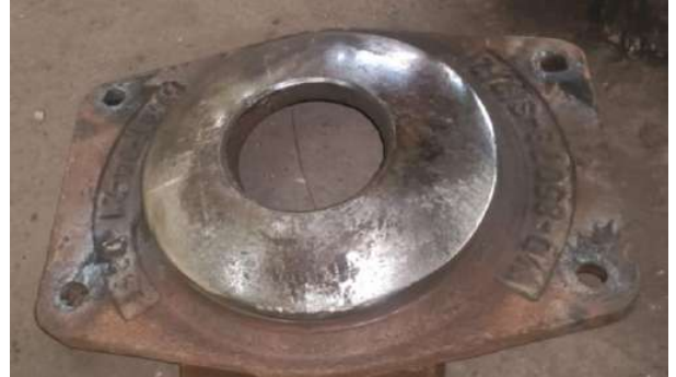
Figure 12 Spherical CP top removal (Rivet/lock bolt shall be cut using gas torch and damage to body bolster should be avoided. Care shall be also be taken to avoid any injury, due to falling of top CP)
