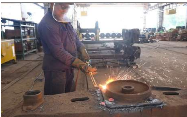
Figure 19 Spherical CP bottom removal (flame shall be pointed towards CP bottom to avoid damage to bolster)
