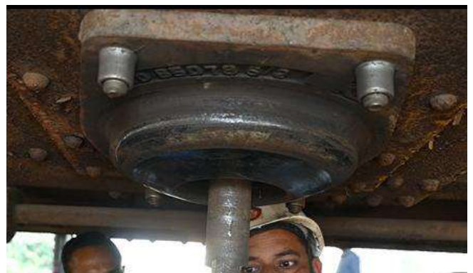
Figure 26 Spherical CP top fitment (two diagonal holding bolts shall be fitted, followed by lock bolting in two holes, removal of holding bolt and lock bolting, one at a time in the remaining two holes)
