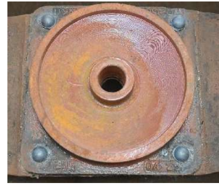
Figure 21 Welding of CP bottom with bogie bolster
