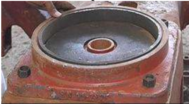
Figure 28 flat CP bottom removal (flame shall be pointed towards CP bottom to avoid damage to bogie bolster)
