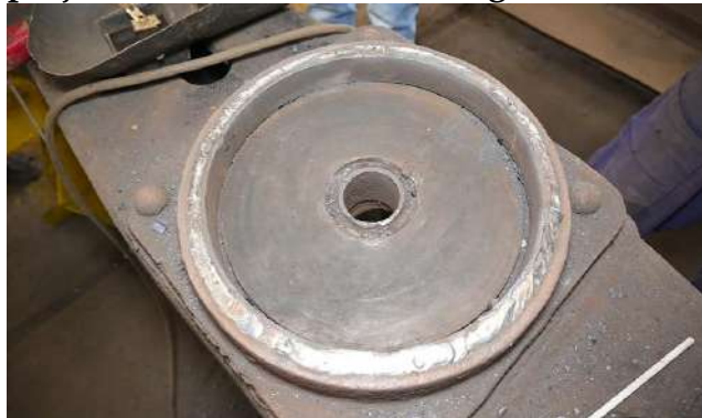
Figure 14 Flat CP- after liner fitment
