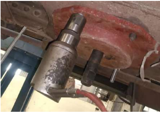
Figure 35 New Flat CP top fitment (Lock bolting shall be done in remaining 04 holes with fitment in diagonally opposite location in sequence, removal of holding bolts and lock bolting in these two holes)
