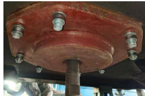
Figure 32 New Flat CP top fitment (Lock bolting shall be done in remaining 04 holes with fitment in diagonally opposite location in sequence, removal of holding bolts and lock bolting in these two holes)
