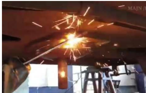
Figure 21 Flat CP top removal (Rivet/lock bolt shall be cut using gas torch and damage to body bolster should be avoided. Care shall be also be taken to avoid any injury, due to falling of top CP)
