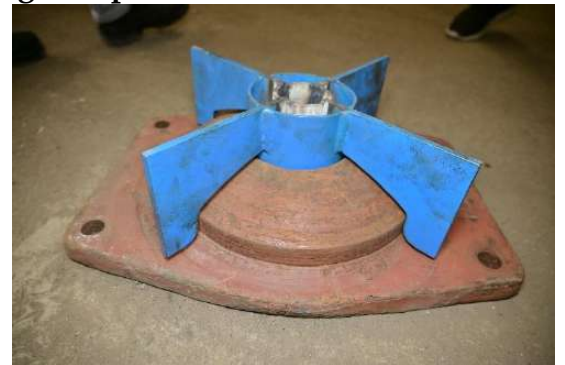
Figure 13 Spherical CP top examination (Gauge no. WD-25094-S/2 should rotate freely over CP top)
