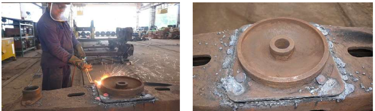
Figure 5 Spherical CP bottom removal (flame shall be pointed towards CP bottom to avoid damage to bogie bolster)
