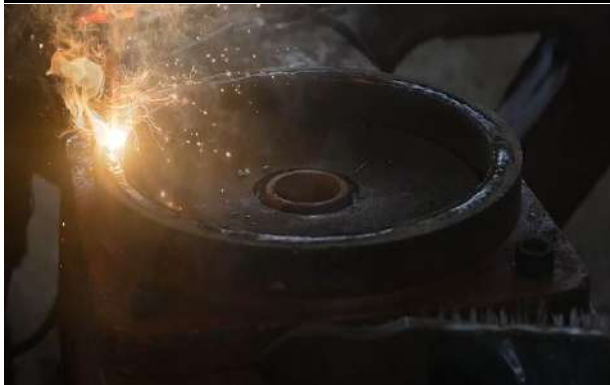
Figure 26 New flat CP bottom fitment with liners (Two bolts shall be fitted diagonally to hold the CP in position, followed by riveting in two holes, removal of bolts and riveting in remaining two holes followed by welding of CP bottom with bogie bolster)
