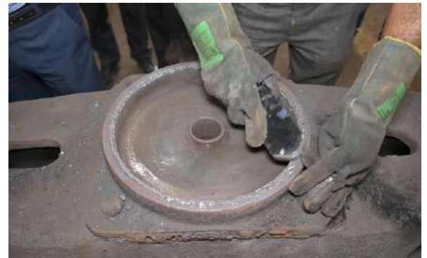
Figure 1 Flat CP bottom cleaning
