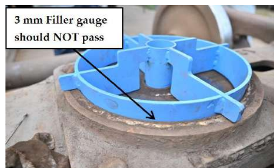
Figure 12 Flat CP- horizontal gauging after liner fitment (gauge should rotate without any obstruction to ensure proper fitment)
