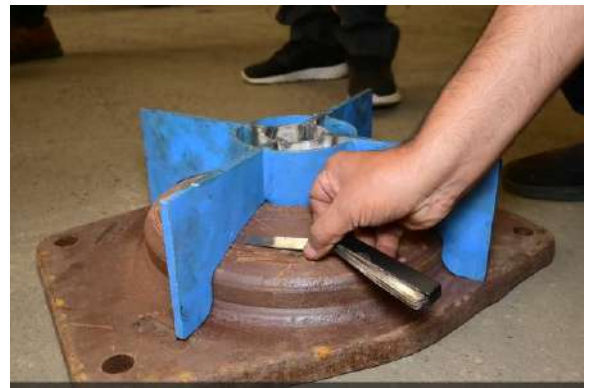
Figure 11 New Spherical CP top gauging before fitment (3 mm filler gauge must not pass at time of fitment)
