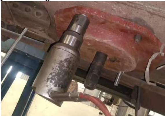
Figure 25 New Flat CP top fitment (Lock bolting shall be done in remaining 04 holes with fitment in diagonally opposite location in sequence, removal of holding bolts and lock bolting in these two holes)
