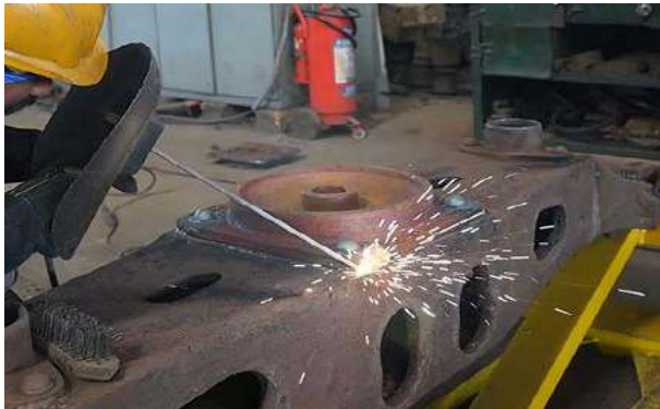
Figure 21 Welding of CP bottom with bogie bolster
