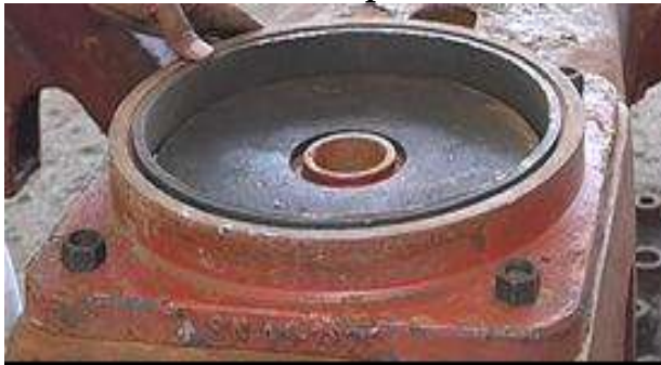
Figure 25 flat CP bottom removal (flame shall be pointed towards CP bottom to avoid damage to bolster)
