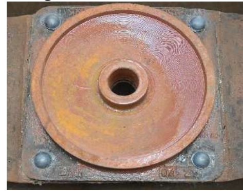
Figure 7 Welding of CP bottom with bogie bolster
