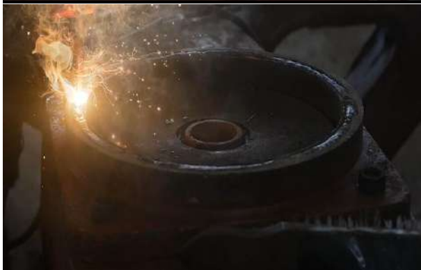
Figure 29 New flat CP bottom fitment with liners (Two bolts shall be fitted diagonally to hold the CP in position, followed by riveting in two holes, removal of bolts and riveting in remaining two holes followed by welding of CP bottom with bogie bolster)
