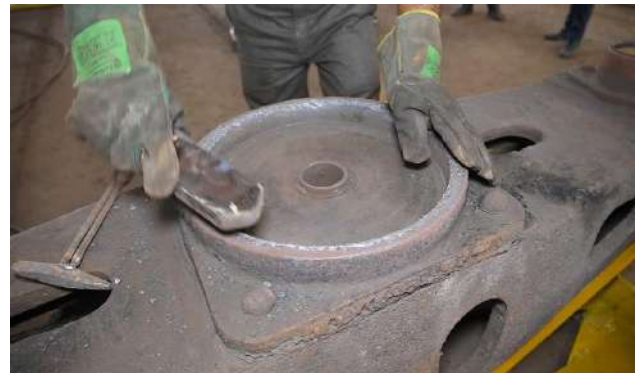
Figure 7 Flat CP- cleaning after liner removal
