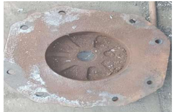
Figure 21 Flat CP top removal (Rivet/lock bolt shall be cut using gas torch and damage to body bolster should be avoided. Care shall be also be taken to avoid any injury, due to falling of top CP)
