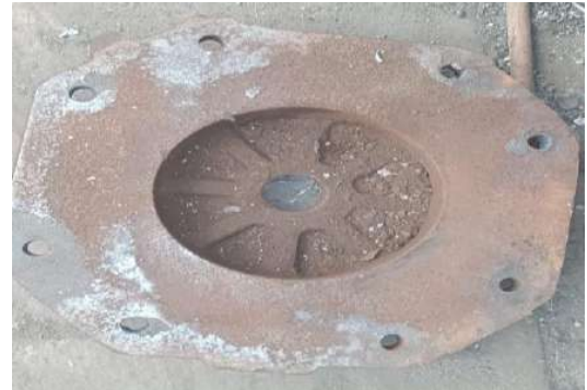
Figure 31 Flat CP top removal (Rivet/lock bolt shall be cut using gas torch and damage to body bolster should be avoided. Care shall be also be taken to avoid any injury, due to falling of top CP)
