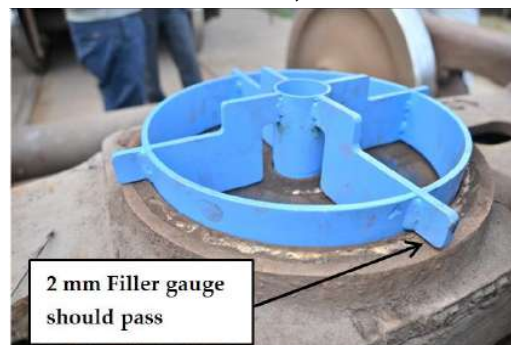
Figure 10 Flat CP- vertical gauging after liner fitment (gauge should rotate without any obstruction to ensure proper fitment)
