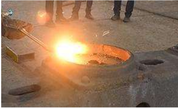
Figure 25 flat CP bottom removal (flame shall be pointed towards CP bottom to avoid damage to bolster)
