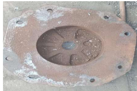
Figure 28 Flat CP top removal (Rivet/lock bolt shall be cut using gas torch and damage to body bolster should be avoided. Care shall be also be taken to avoid any injury, due to falling of top CP)
