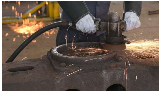
Figure11 Flat CP- grinding after liner welding
