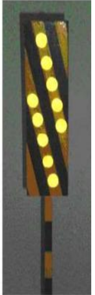
Passenger warning board
