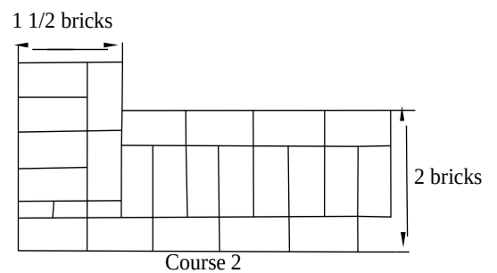
1 1/2 BRICK WALL JOINING 2 BRICK WALL
