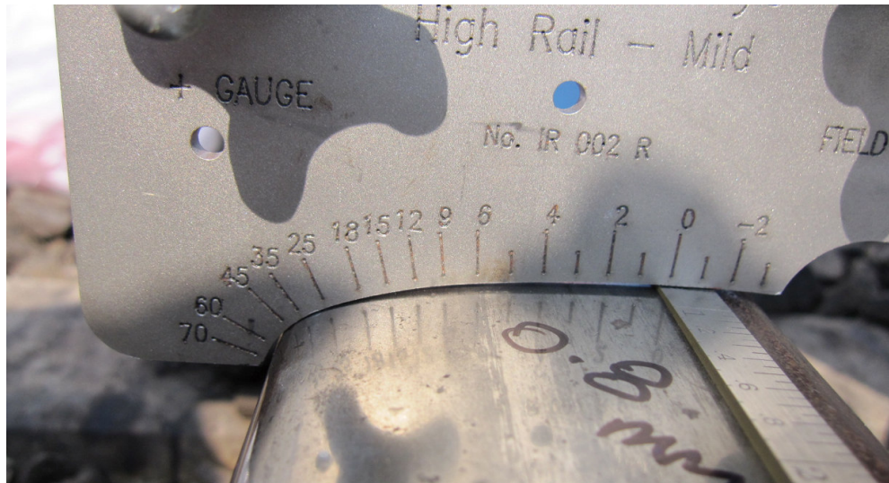
Fig. 23: Measurement Using BAR GAUGE
