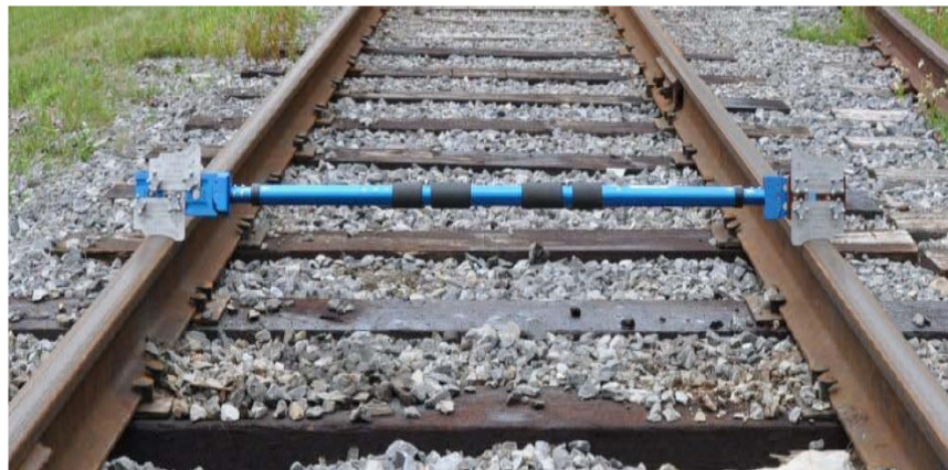
Fig. 22: BAR GAUGE Having Four Templates
