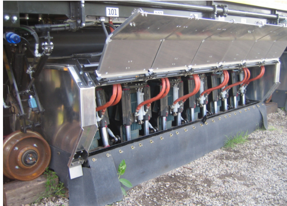
Fig. 5: Grinding Motors on a Buggy
